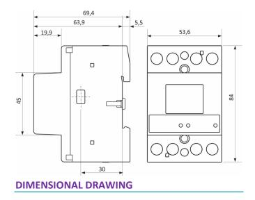
Figure 3: Dimensional drawing of 3MEM40-EVR
