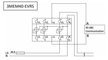
Figure 2: Single-phase connection diagram
