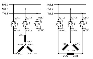
Figure 3.11: SSW900 with standard connection
