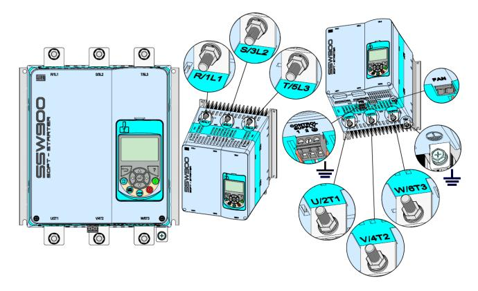
Figure 3.6: Power and grounding terminals, frame C
