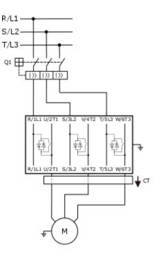
Power supply connection: R / 1L1, S / 3L2 and T / 5L3 At the top of the SSW and left side of the thyristor bridges.
