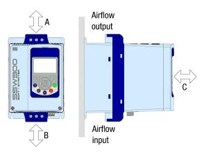
Figure 3.2: Clearances for ventilation
