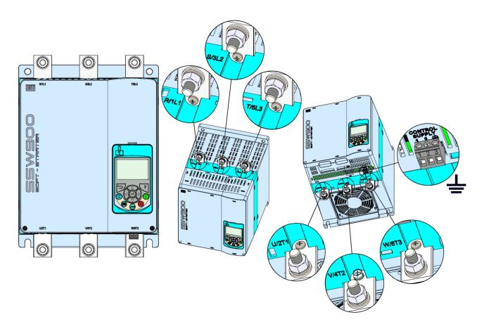
Figure 3.7: Power and grounding terminals, frame D
