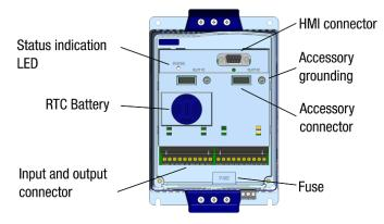
Figure 2.2: Access to the control of the SSW900
