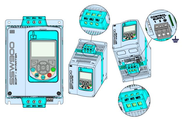
Figure 3.4: Power and grounding terminals, frame A
