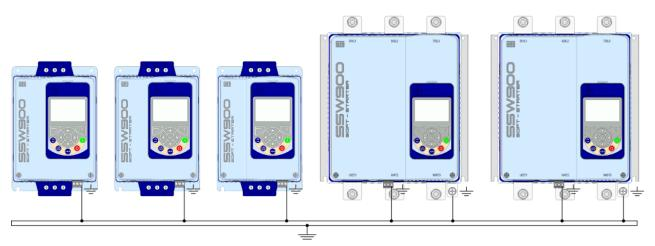
Figure 3.14: Grounding connections for more than one SSW900
