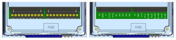
Figure 3.17: Position of the connections on the control board
