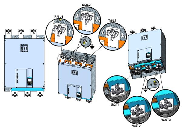
Figure 3.10: Power and grounding terminals, frame G
