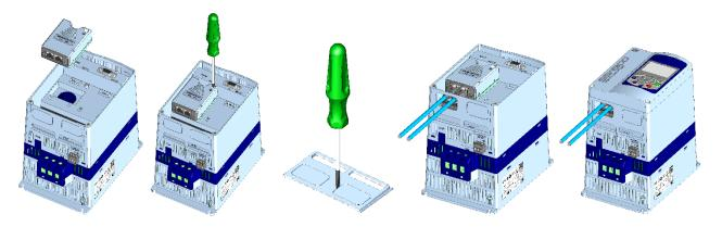
Figure 6.1: Procedure to install accessory
