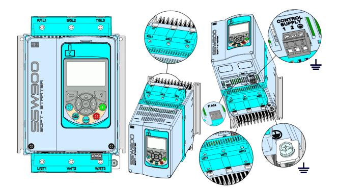
Figure 3.5: Power and grounding terminals, frame B
