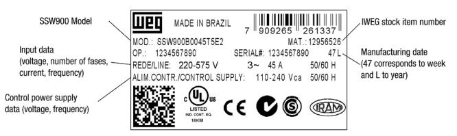
Figure 2.3: Soft-Starter SSW900 identification plate
