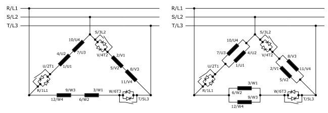
Figure 3.13: SSW900 inside delta motor connection with double delta
