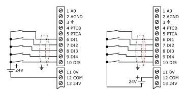
Figure 3.19: Wiring diagram of the digital inputs using external power supply
