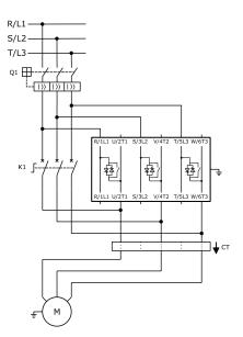
Figure 8.9 External Contactor Connection Scheme
