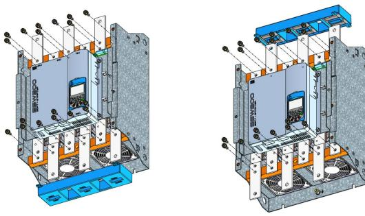
Figure 8.5: Removing the busbars and CT'
